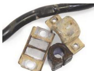
Figure 2 - the anti roll bar, brackets and the original rubber bush
